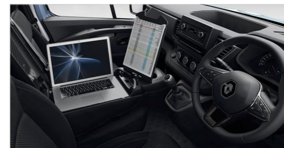
8. Work station centre seat
